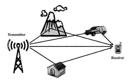
Figure 2.1 Concept of wireless multipath channel
