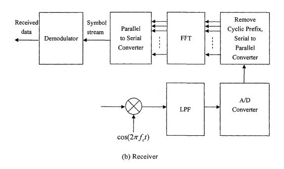
Figure 2.3 Block diagram of an OFDM system
