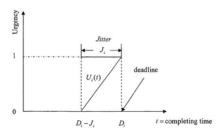
Figure 4.2 Concept of jitter for RT traffic
