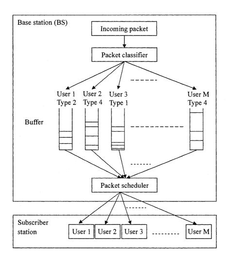
Figure 3.1 Architecture of packet scheduling algorithm
