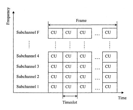
Figure 3.2 OFDMA channel structure
