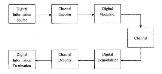
Figure 2.2 Basic structure of a digital communication system
