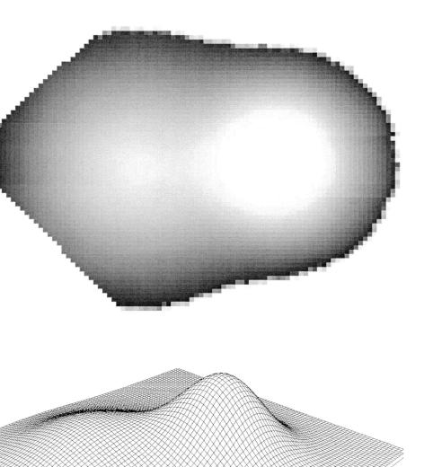
Figure 4 - Simulated bivariate probability density field, in two dimensions. The probability field is derived from a sum of two normal curves. (a) shows a orthographic (map) view, using brightness to indicate increasing density. (b) shows a simulated perspective view of the same field.
