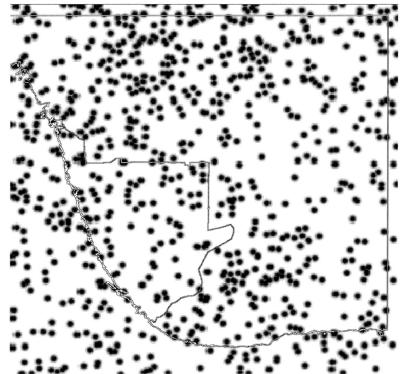
Figure 11 - Probability density map of positive polarity lightning strikes. The values in the map represent the relative likelihood of a strike having happening in that area in the study period. Increasing probability is indicated by an increased intensity of black.
