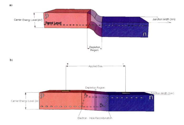
1.2: a) A p-n junction with pink and blue colours representing hole and electron concentrations respectively. b) When under bias, minority carriers drift and diffuse across the junction, producing light when they combine with majority carriers.
