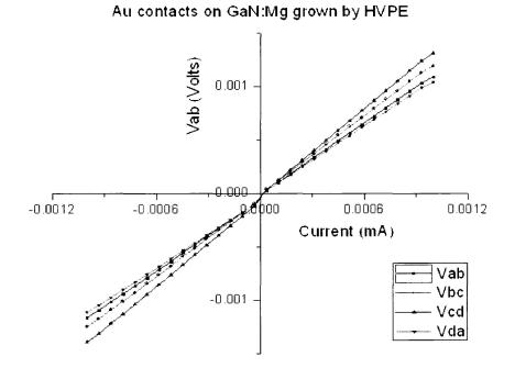
Figure 3.15: Small signal measurement of the I-V response of gold contacts on GaN:Mg. A small,  $\pm 1.2\mu A$  sweep of current exposes even small rectifying behaviour. As is visible from the slight nonlinearity near the origin, the contacts had a built-in potential of around 0.1mV, which is small enough for any measurement in this work.
