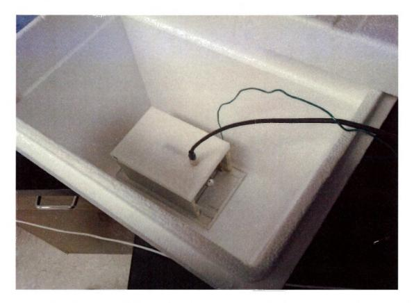
Figure 3.17: The placement of the Hall system in a thermally insulating styrofoam container.Table 3.3: The carrier concentration of GaN:Mg grown by HVPE measured at high and low temperatures in a thermally insulating container. Negative carrier concentrations imply a
