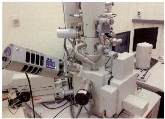
Close up of scanning electron microscope
