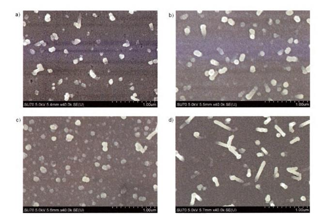
Figure 4.6: Surface SEM images of magnesium doped GaN samples grown by low temperature MEAglow. Films were grown at a) 545°<sup>C</sup>, b) 580°<sup>C</sup>, c) 600°<sup>C</sup>, and d) 635°<sup>C</sup>. In addition to metal droplets, there is the presence of nanowires.
