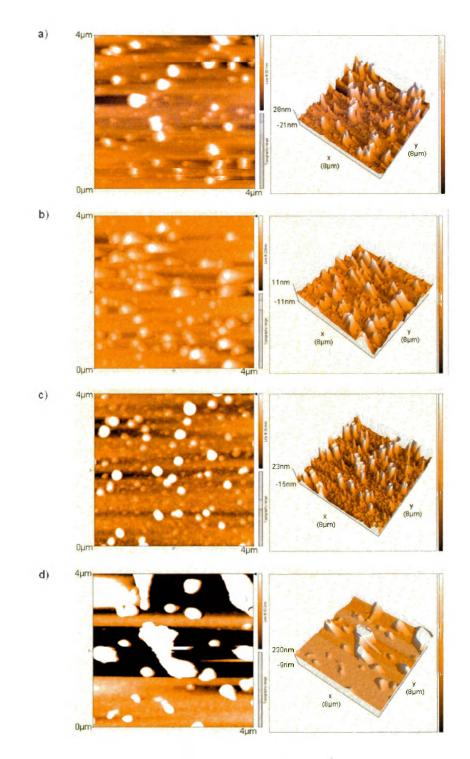
Figure 4.12: AFM images of the magnesium doped GaN films grown using low temperature
