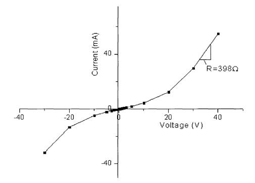
Figure 5.2: The I-V characteristics of the InGaN p-GaN LED. The series resistance measured in the flatband configuration was 398 $\Omega$ , although this value could be underrepresented because of the surface n-oxide resting on the p-GaN.
