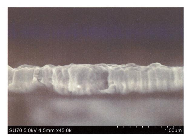
Figure 4.9: SEM image of InN grown by MEAglow. Here, the vertical columnar structure is evident.
