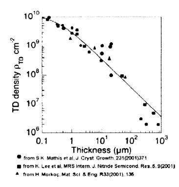
Figure 2.5: A summary of research into the dislocation density as a function of buffer layer thickness. Plot taken from [28].
