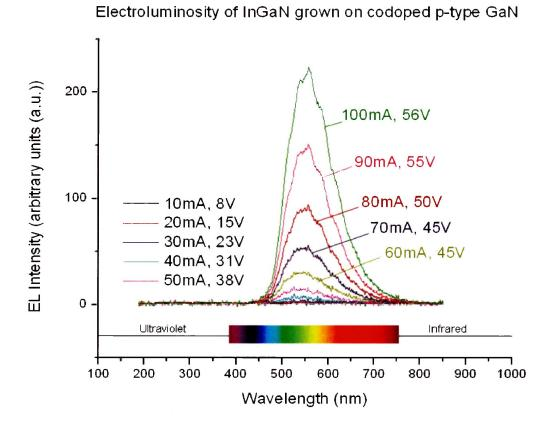
Figure 5.5: The measured electroluminosity of InGaN grown on a codoped p-type GaN template. Here, the peak lies in the green - yellow region.
