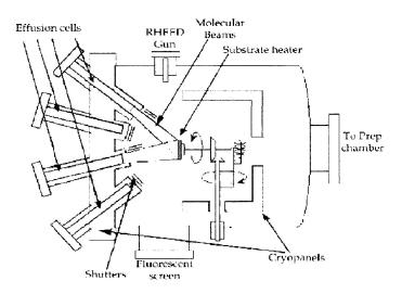
Figure 2.9: The makeup of an MBE system. Effusion cells emit beams of atoms toward the surface of the substrate where upon contact they form the GaN lattice. Picture taken from [47]
