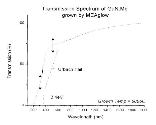
Figure 4.17: The absorption spectrum of a sample of GaN showing the Urbach characteristic. The surface oxide causes absorption to occur at values not exactly equal to the 3.4eV bandgap.
