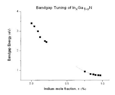
Figure 5.6: The bowing of bandgap energy of an InGaN alloy (graph modified from [74]). Here, there is a nonlinear interpolation of the bandgap energy between low gallium content (indium rich) and high gallium content (gallium rich) films.
