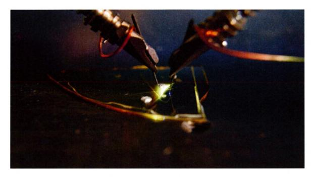
Figure 5.4: A picture of the InGaN on codoped p-GaN LED during operation. One side of the film (the right side) had a cover placed on top during growth so that it is exposed to the surface. Two electrodes can thus contact each side of the p-n junction, allowing light to emanate. Picture was taken with a high exposure time (30s).
