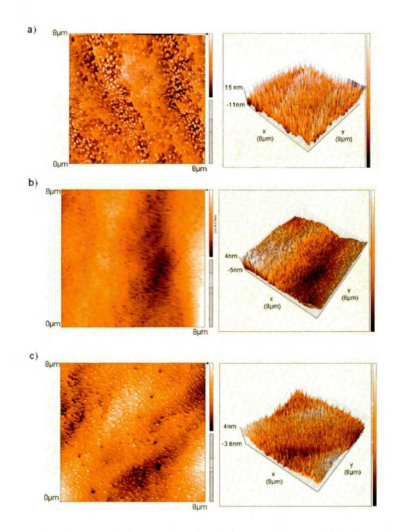
Figure 4.11: AFM images of a) magnesium doped, b) undoped, and c) silicon doped GaN grown by HVPE. Samples doped (with either silicon or magnesium) showed many surface defects, whereas the undoped sample showed terracing.
