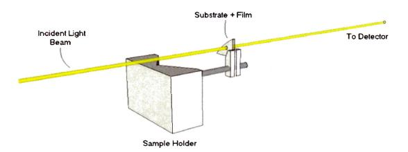
Figure 4.14: The probing of the spectrophotometer. A sample holder places the film toward the light beam and the detector measures the attenuated beam.
