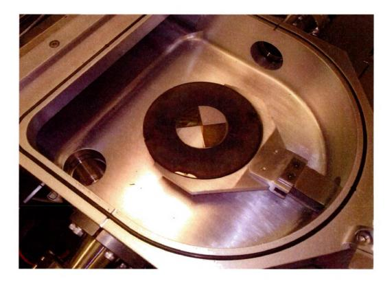
Figure 4.3: The placement of the sapphire substrates (clear 4 wafer sections) in proximity to the surrounding aluminum disk and extra sapphire covers (discarded GaN samples, dark 4 wafer sections). The configuration is expected to act to lower temperature and prevent atomic deposition from the sample holder.
