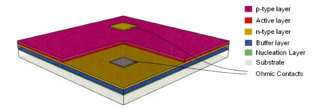
Figure 2.1: An LED formed in a Mesa structure. Here, a forward bias is applied to the p-type and n-type layers through their ohmic contacts, transporting charge across the active layer.
