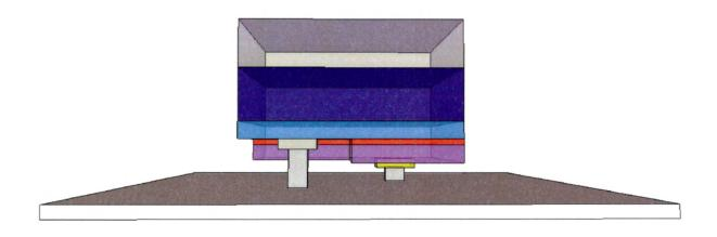
Figure 2.15: The flip chip configuration. Here, light produced by the active layer reflects off the bottom plane, increasing the luminosity.
