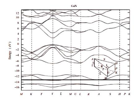
Figure 4.13: The calculated band structure of gallium nitride. The minimal energy transition between the  $\Gamma$  apexes is known as the bandgap (3.42eV). The Brillouin zone used for the calculation is also included. Figure taken from [44].
