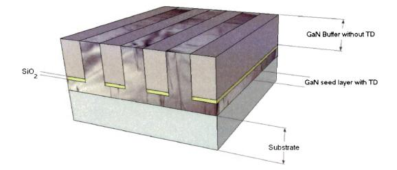
Figure 2.6: The principle of the Lateral Epitaxial Overgrowth method. The application of a dielectric mask decreases the threading dislocations in the mask overgrowth by preventing threading dislocations from protruding farther into the film.
