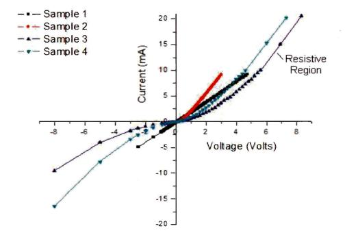
Figure 3.19: I-V response of four samples of GaN:Mg grown by MEAglow on GaN:Si grown by HVPE. Here, electrodes contacted the ohmic gold pad on the p-side and the ohmic indium-tin pad on the n-side. Characteristics were heavily dominated by series resistance, especially sample 1 which showed no rectification.
