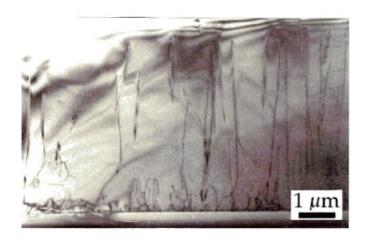
Figure 2.2: Threading dislocations protruding upward from the sapphire substrate located at the figure's bottom. Image is of a Transmission Electron Microscope (TEM) taken from [23].
