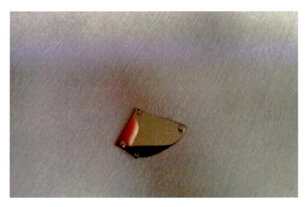
Figure 3.16: p-type germanium Hall sample with annealed indium-tin contacts.
