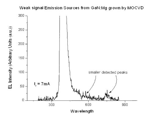
Figure 3.6: Weak emission sources from current passing through two terminals placed on the surface of GaN:Mg grown by MOCVD. There is an evident harmonic at 750nm, and a questionable source at ~580nm (yellow).
