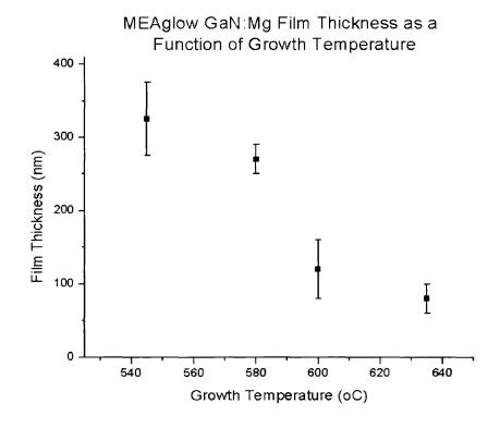
Figure 4.7: A plot of the film thickness versus the growth temperature. The graph shows a downward trend. Error bars were estimated from the individual images themselves.
