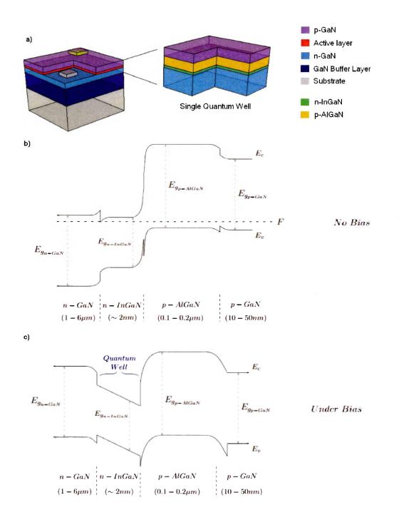
Figure 2.13: The single quantum well and it's a) physical structure, b) band diagram, and c) band diagram under forward bias. Band structure reflects the Anderson model to demonstrate the offsets between each material. Material thicknesses were obtained from reports in [14] for the leftmost three materials, and the p-GaN thickness is derived from observation in the lab.
