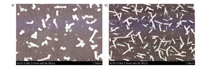
Figure 4.8: Surface SEM images of two samples that had uncharacteristically large densities of nanowires as compared to their counterpart samples, grown at the same temperature: a) Sample grown at  $545^{\circ C}$  and b) sample grown at  $635^{\circ C}$ . The counterpart samples in question are Figure 4.6a and 4.6d respectively.
