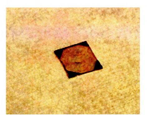
Figure 3.14: : Preparation of a magnesium doped GaN sample for Hall measurements. First the section is annealed in  $H_2O$ : HCl, then gold is sputtered on the corners of the section, and finally it is annealed in a vacuum for 60 minutes.
