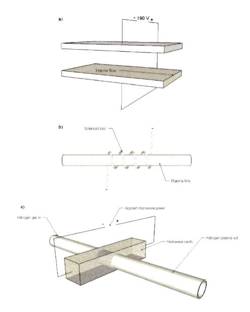
Figure 2.10: Three architectures of plasma sources. a) Capacitive, b) Inductive, c) Microwave
