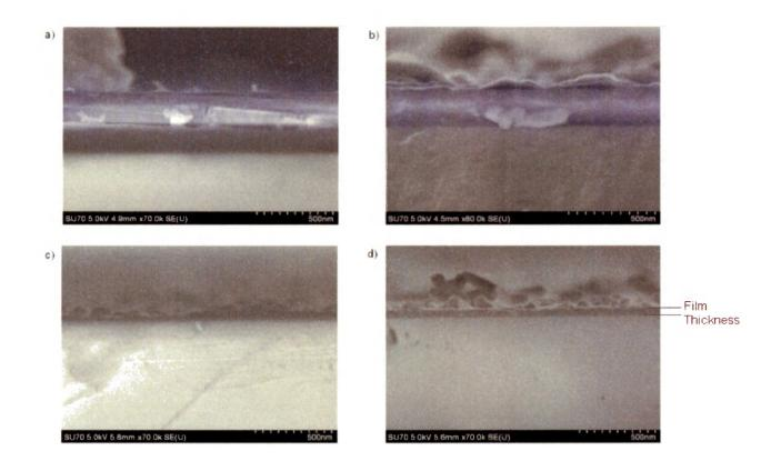
Figure 4.5: Cross sectional scanning electron microscope images. Films were grown at a) 545°C,
