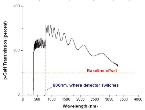
Absorption Spectrum of Magnesium Doped GaN grown by HVPE
