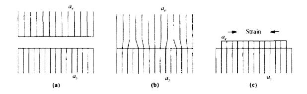
Figure 2.4: A depiction of an epitaxial layer atop a substrate, both with different lattice constants, a<sub>e</sub> and a<sub>s</sub> respectively. a) before interlacing occurs, they maintain expected lattice spacing. b) after interlacing, dislocations become present. c) In between dislocations, the atoms of one of the epitaxial layer strains to match that of the substrate, with the outer atoms experiencing more strain. Figure taken from [27].
