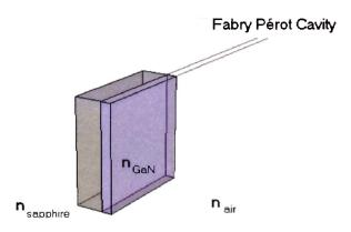
Figure 4.16: The formation of a Fabry-Pérot cavity from the GaN film. Light passing through the sapphire and then the GaN film resonate between their boundaries, forming interference
