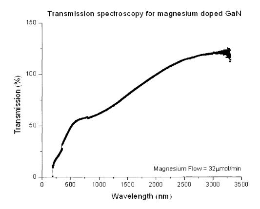
Figure 4.21: The transmission spectrum of a magnesium doped GaN sample grown by low temperature MEAglow with a smaller  $CP_2Mg$  flow. The change in the system caused sample defects which increased the attenuation, causing the bandgap to be measured incorrectly.
