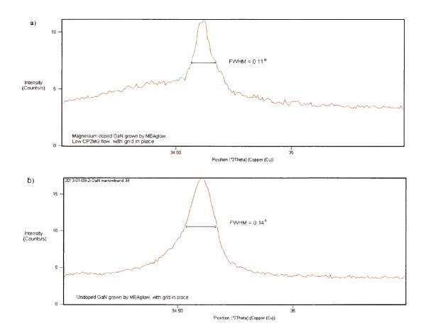
Figure 4.23: X-Ray diffraction measurements of a) magnesium doped GaN grown at 600°<sup>C</sup> with lower CP2Mg flow and the reconfigured plasma source, and b) undoped GaN grown at 600°<sup>C</sup> with no CP2Mg flow and the reconfigured plasma source. Both show the presence of a sharp peak due to GaN nanowires. The diffraction intensity for the magnesium doped sample was close to that found from samples grown without the RF shield, however the undoped sample had a lower intensity.
