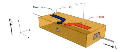
Figure 3.7: The Hall measurement of a bar sample. Here, current pumped in the x direction is curled toward the terminals located on the x-z surfaces to generate a detectable Hall voltage.
