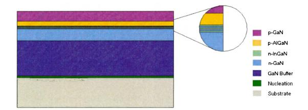
Figure 2.14: The Multi Quantum Well structure (MQW). Here, any carriers that would not be trapped within a single quantum well would likely be confined by the other wells.
