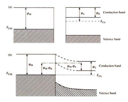
Figure 3.10: A Metal-Semiconductor junction and its resulting band deformation upon contact. Figure taken from [58]. a) Before contact is made. Each material has their own Fermi level or metal work function, and hence the bands are horizontal. b) Upon junction, these levels equate, and their difference is approximately equal to the potential difference between the two individual levels.
